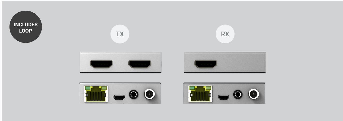
A compact, palm-sized HDMI 2.0 extender set - supports 18Gbps premium UHD/4K 60Hz 4:4:4 data rates, with all current HDR formats inc. Dolby Vision®, HDR10 and HLG up to 40 metres, over one twisted pair Cat cable.
